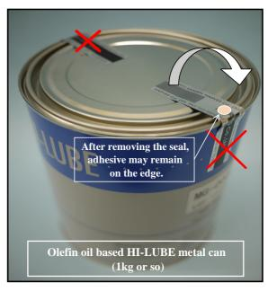
\*. If you insert lubricator plate, adhesive may contaminate the grease.
